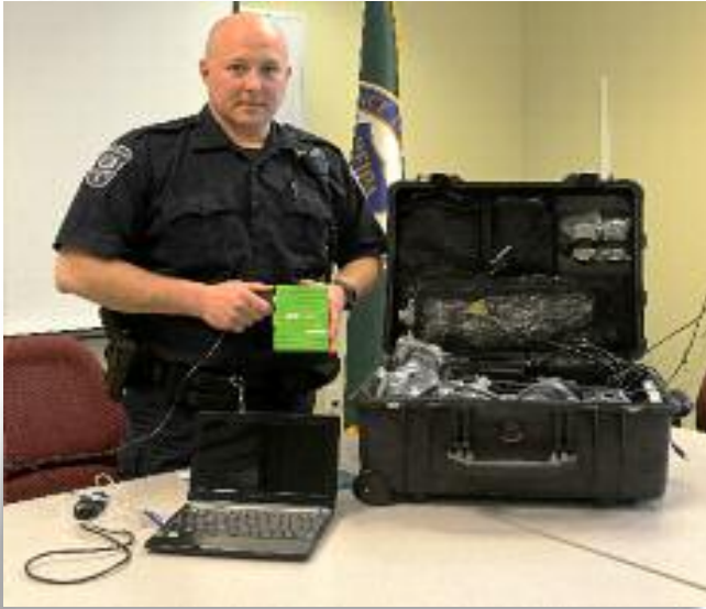
Cst. Ron Kennedy, a traffic specialist with Charlottetown Police Services displays a crash data recovery system now in use by the department. It reads data collected and stored by a vehicle's airbag restraint system which can include vehicle speed, brake activation time and force, antilock brake activation, seatbelt engagement and many other points of data.
